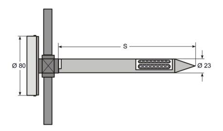
The hygrometer for pricking is mainly used in agriculture to define the moisture content of corn. The hygrometer is insensible to its position and can be used axial, vertical or in oblique position.
